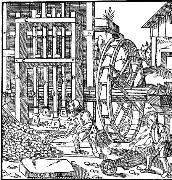
Illustration of a Stamper Mill. (Note, the mechanism of a stamper mill is much like that of a fulling mill, only the stampers are replaced with mauls)
